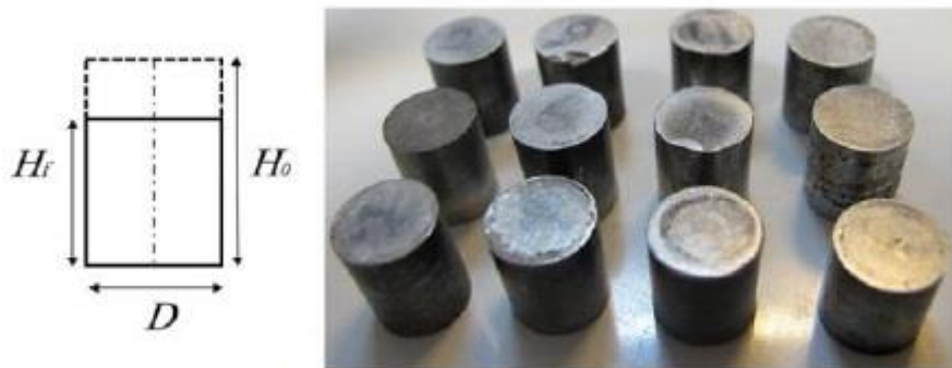
Fig. 7 Hot pressed powder samples and their main dimensions
